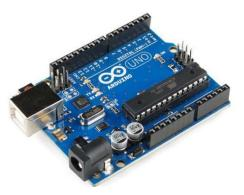
Figura 01 – Arduino Uno Fonte :http://www.hobbytronics.co.uk/
